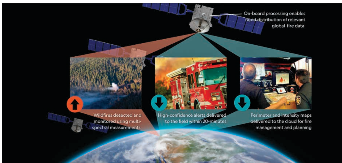
Rendering of a low-earth orbit satellite system optimized for wildfire detection and tracking, courtesy of Environmental Defense Fund.
