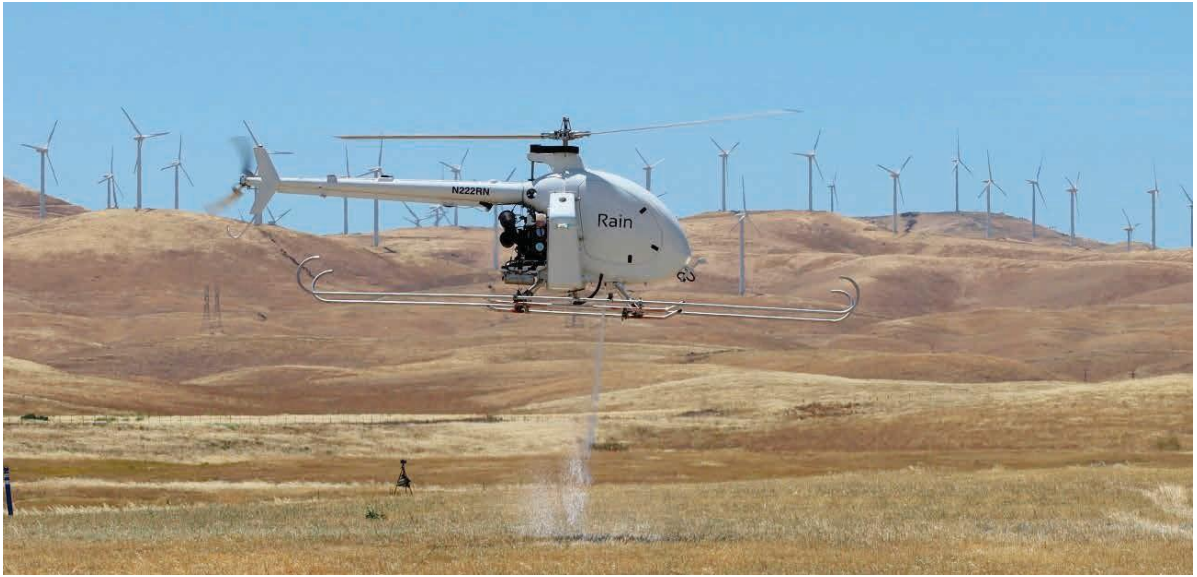
Figure 6. The Rain MK2 Aircraft being tested to rapidly contains wildfire ignitions in San Mateo County
